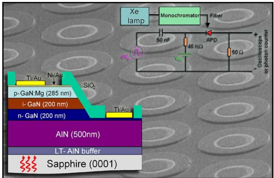
**Figure Caption:** Lower left, schematic diagram of a back illuminated single photon detector; Upper right, biasing circuit used to drive the single photon detector; Background, scanning electron micrograph of a processed array of single photon detectors.
