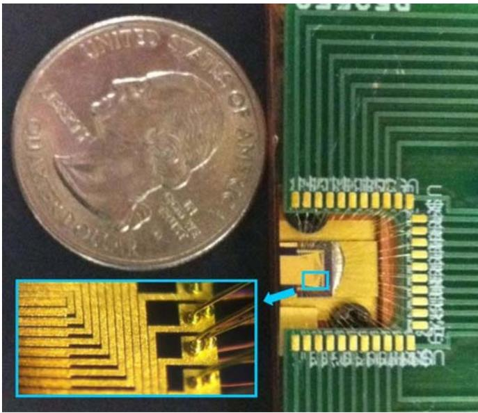
**Figure 1.** Fully packaged distributed feedback quantum cascade laser array compared with a US quarter. This device can operate in continuous-wave mode with a wavelength coverage of 4.5–4.7 $\mu\text{m}$  at room temperature.
