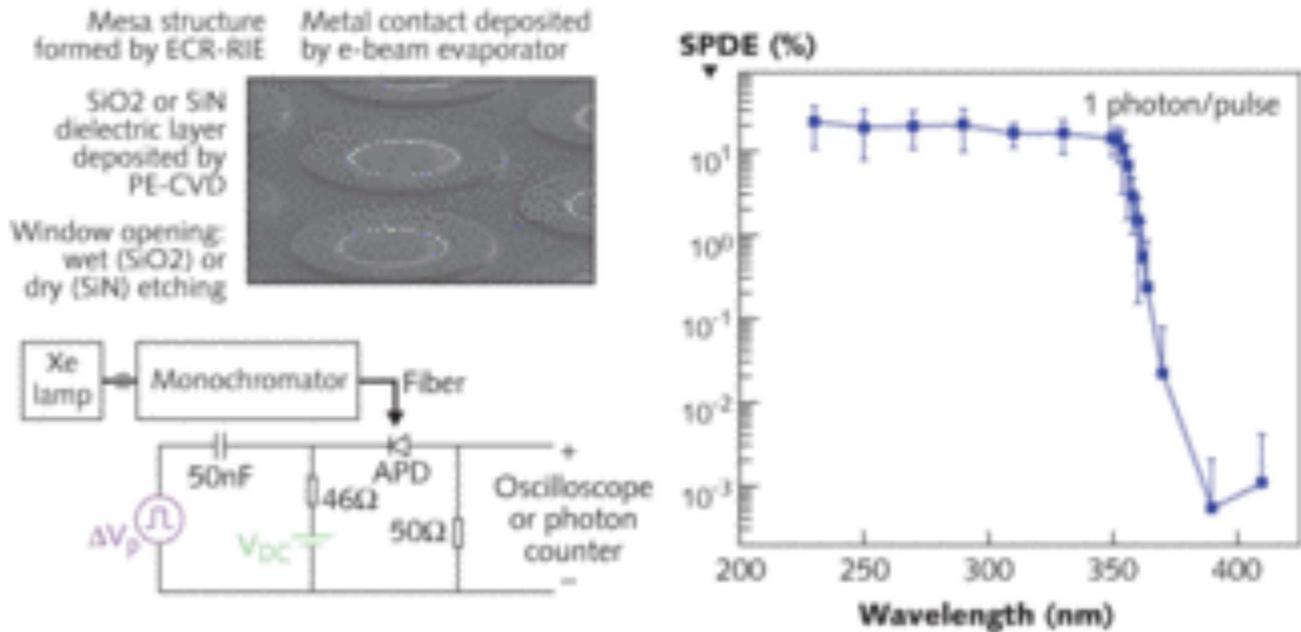
FIGURE 4. A fabricated GaN APD (upper left) uses pulsed quenching circuitry (lower left) for Geiger-mode operation. SPDE varies according to the wavelength of the photon source (right).
