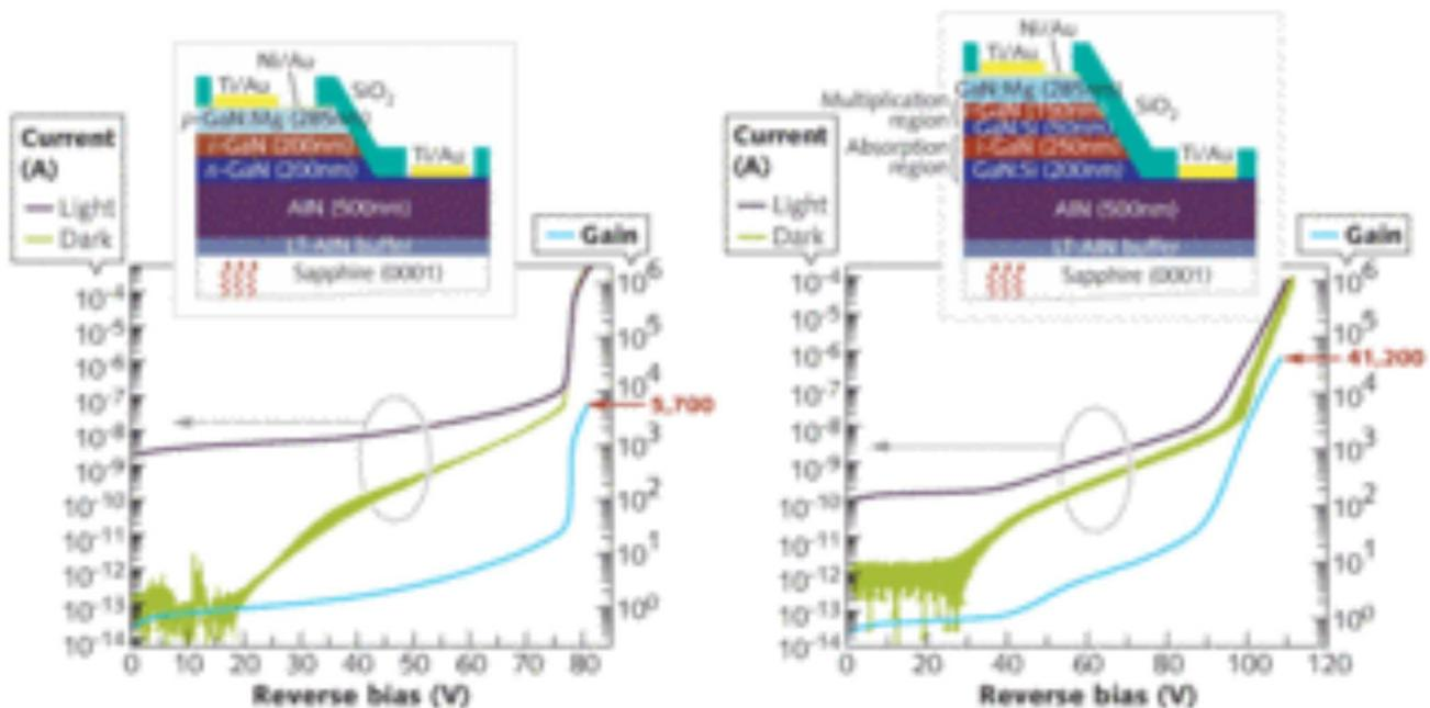
**FIGURE 1.** Traditional PIN APD devices (left) don't measure up to SAM-APD devices (right), whose gain enhancement is made possible through the use of the separate absorption and multiplication (SAM) regime.
