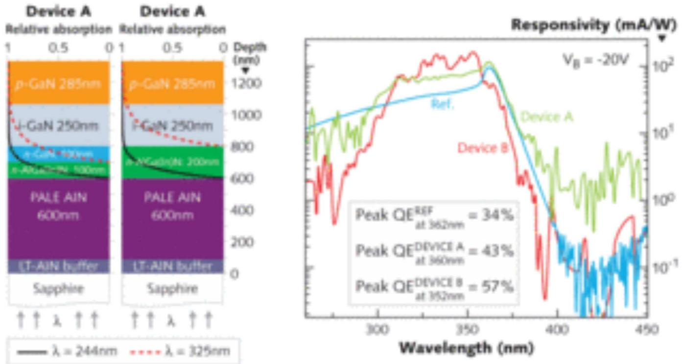
**FIGURE 3.** A back-illuminated PIN APD uses 100-nm-thick GaN on 100-nm-thick AlGa(In)N (Device A), and 200-nm-thick AlGa(In)N as an n-layer (Device B). The quantum-efficiency and responsivity curves of a reference device using 200-nm-thick GaN compares with an APD using AlGa(In)N.
