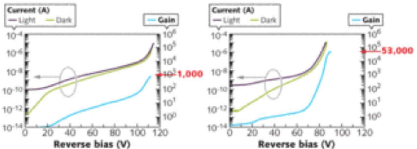
FIGURE 2. Introducing -doping reduces breakdown voltage and increases gain in linear mode, as shown by comparing conventional bulk- (left) and -doped (right) SAM-APDs.
